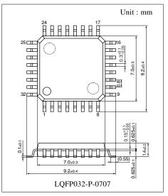
Note) The package of this product will be changed to lead-free type (LQFP032-P-0707B). See the new package dimensions section later of this datasheet.
